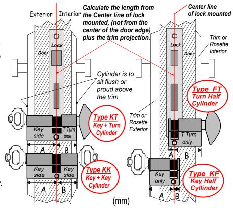
The Euro Profile Cylinder uses the key tip to integrate / drive the internal plunger to work with the cylinder cam. When key is duplicated, make sure that the key tip is made to the same shape and length as the original 'Baton' key furnished. Failure to follow these specifications could wear out the construction and cause malfunction.
